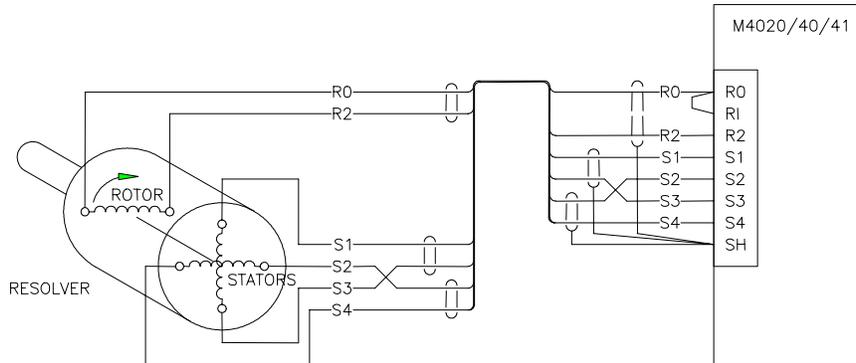
**Figure 12.7 – M1771-4021 Resolver Interface (Stand Alone)**
