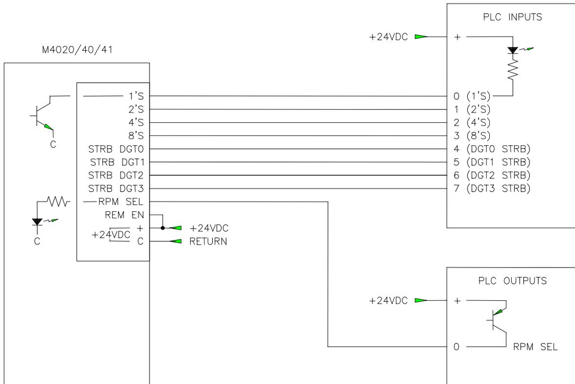
**Figure 9.3 – RPM/Position Output Connector Wired to PLC**
