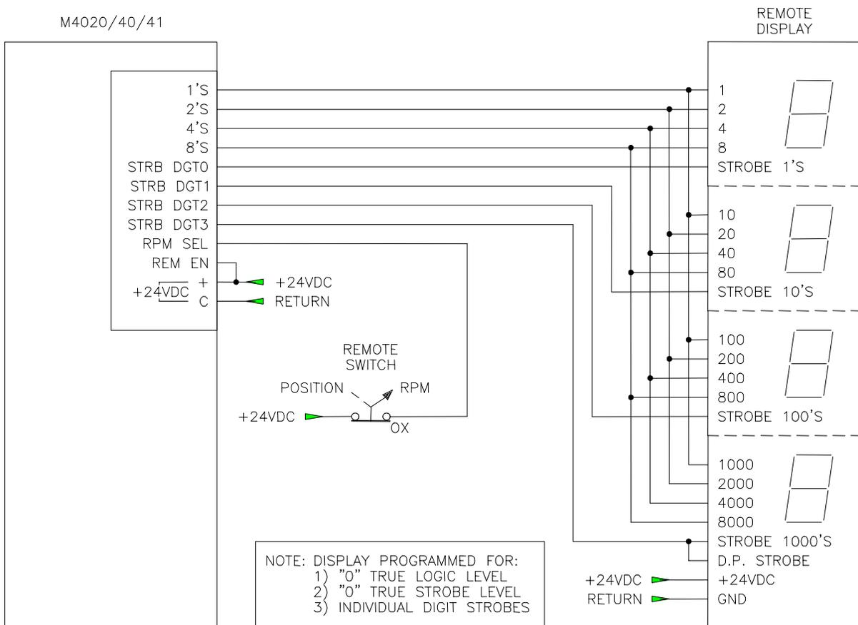
**Figure 9.2 – RPM/Position Output Connector Wired to Remote Display**
